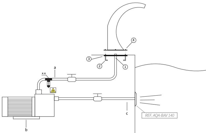
\*\*AQA recommends to install a POOL PROTECTOR to avoid corrosion of the existing stainless steel elements in the pool.
